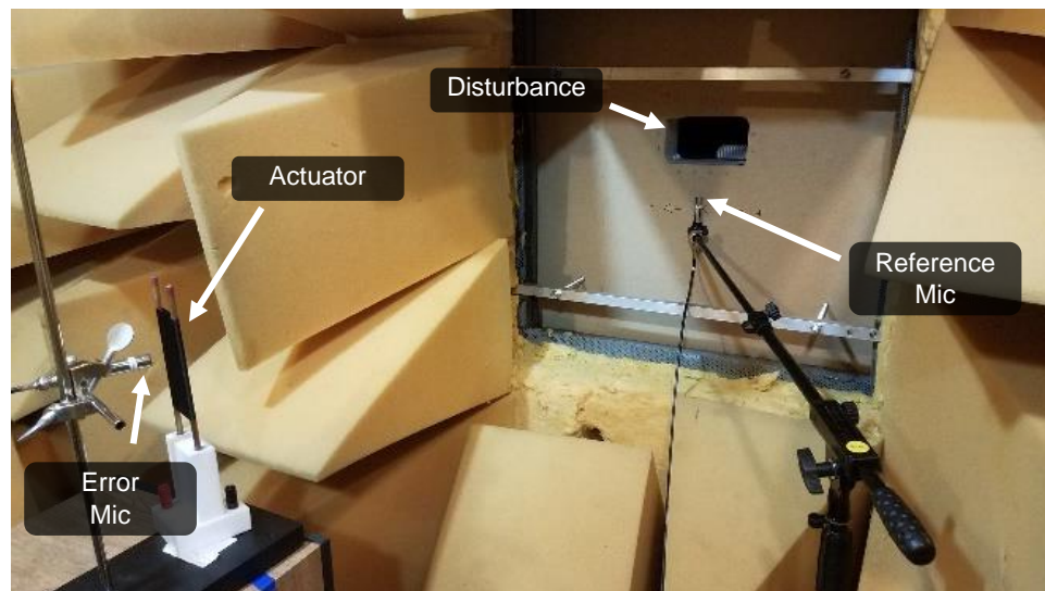
Figure 45: Microphone, Disturbance, and Thermophone Actuator Placement for Free-Field ANC Tests Performed On Blower Fan Noise with the Tiger WIFI-S Controller
