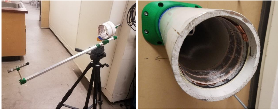
Figure 103: Annular Teflon Speaker in Two Test Configurations
