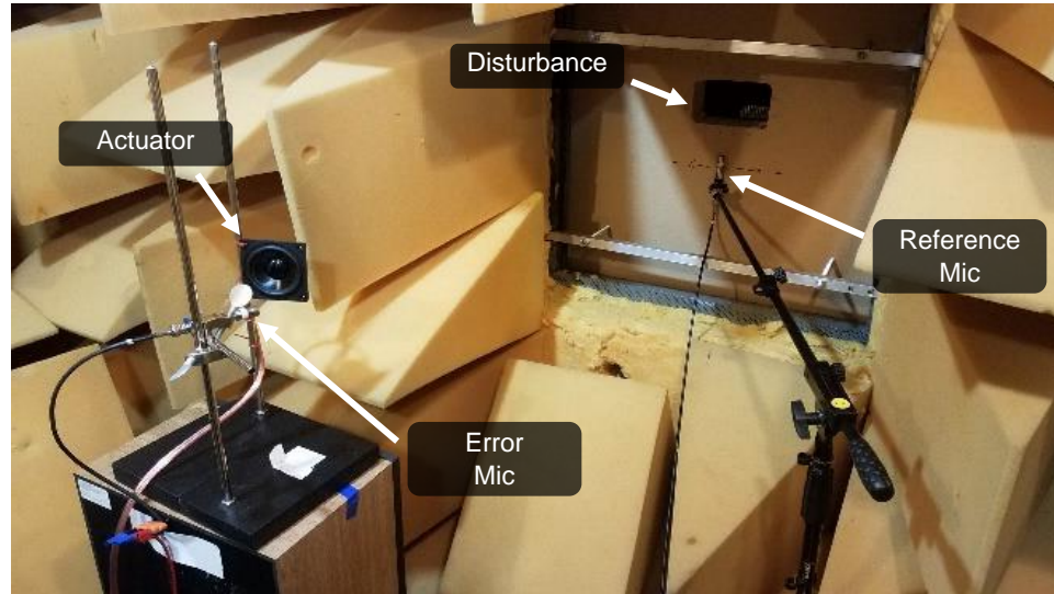
Figure 44: Microphone, Disturbance, and Loudspeaker Actuator Placement for Free-Field ANC Tests Performed On Blower Fan Noise with the Tiger WIFI-S Controller
